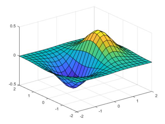
Both the surf function and its companion mesh display surfaces in three dimensions. surf displays both the connecting lines and the faces of the surface in color. mesh produces wireframe surfaces that color only the connecting lines.
