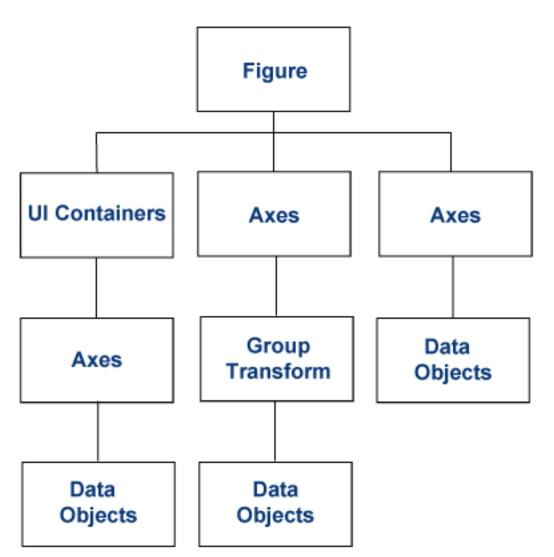
When you call a plotting function, MATLAB creates the graph using various graphics objects, such as a figure window, axes, lines, text, and so on. Each object has a fixed set of properties, which you can use to control the behavior and appearance of the graph.
